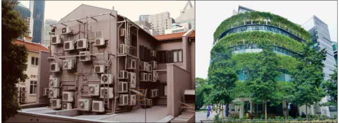
Figure 3. Two buildings in Singapore They represent different urban heat island mitigation and adaptation designs and measures. The one on the left reacts with technology, the one on the right adds green facades and an open first floor.
