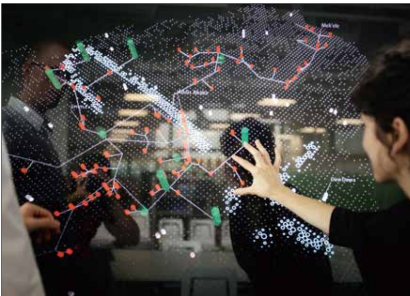
Figure 5. Using a digital geometry abstraction of Ethiopia and its power grid. Programmed for a multi-touch display surface, it serves as an interactive design tool. Settlements are shown in red, power plants in green and the grid connecting them in white. Program development Eva Friedrich, image Carlina Teteris 2013.
