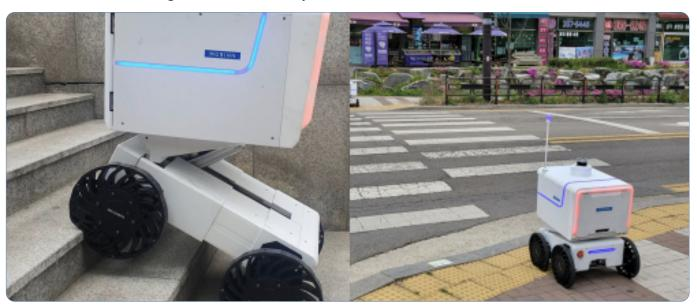
${\color{blue} \blacktriangle}$  An autonomous delivery robot carrying goods is crossing a pedestrian walkway.
