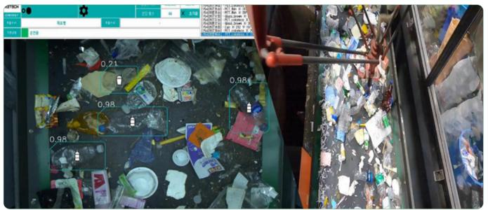
▲ The Al-Based Waste Sorting Robot identifies different types of waste on the conveyor belt, then suctions and transfers recyclable PET plastic bottles. Source: AETECH
