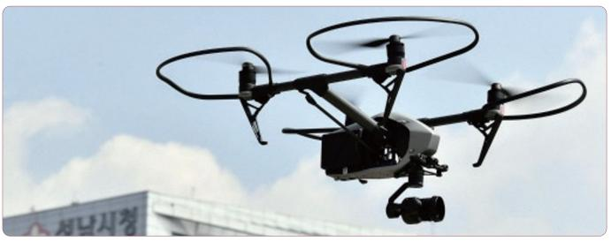
lacktriangle A drone equipped with CCTV video equipment is being deployed to the disaster site.
