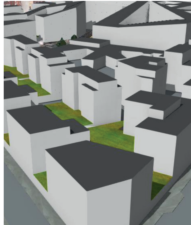
In general, planned building have been modelled with flat roofs and without windows. View from the OpenCities Planner browser-based application, where the models of the planned buildings have been embedded
