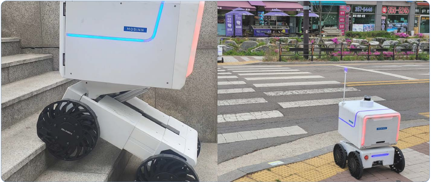
▲ An autonomous delivery robot loaded with goods is crossing a pedestrian crosswalk.
