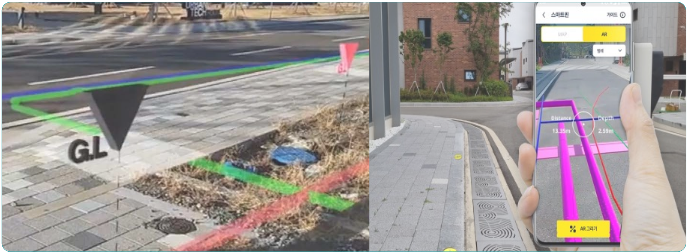
▲ A facility manager views augmented reality-based 3D underground utility locations and attributes.
