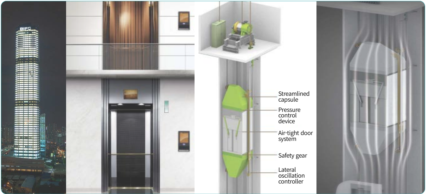
▲ The “streamlined capsule cage” of the ultra-high-speed elevator minimizes operating noise.
