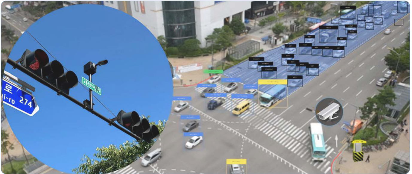
▲ The Intelligent Intersection Management System identifies vehicles using the intersection and analyzes traffic volume.
