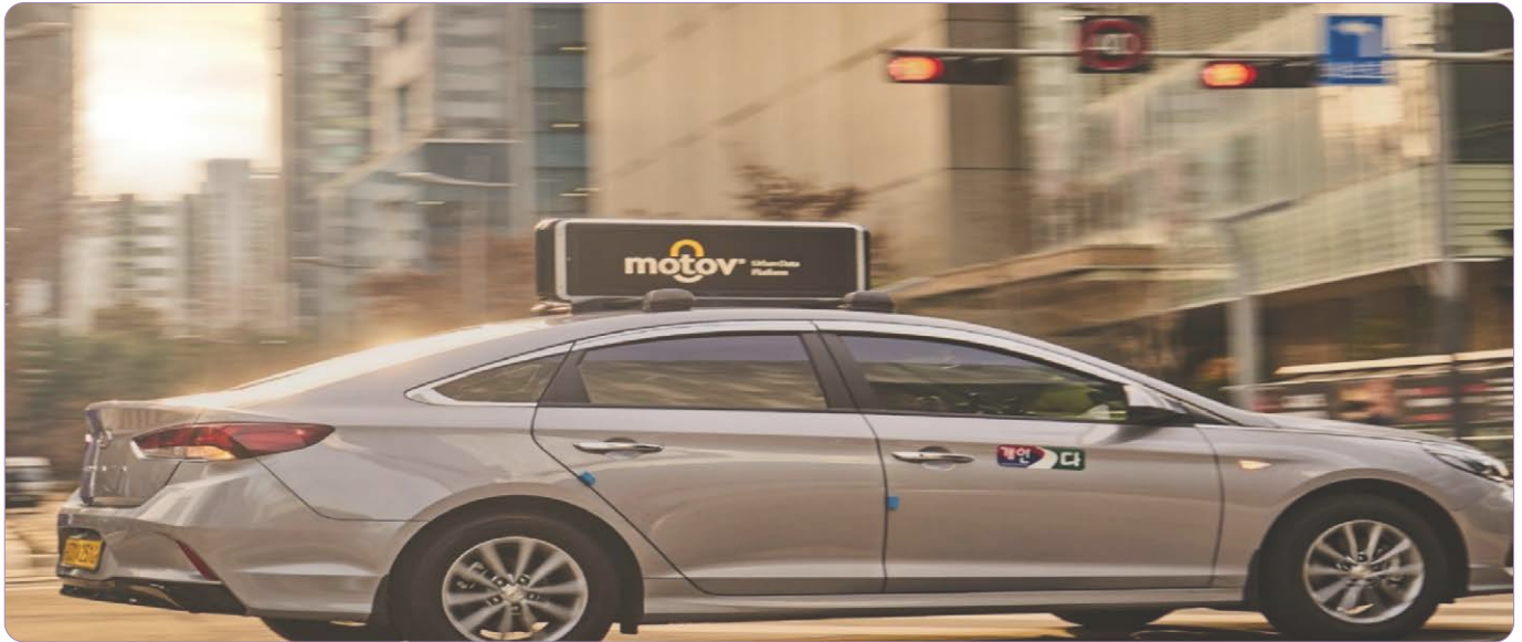
▲ A sensor-equipped device (media board) installed on the taxi roof is collecting urban data.
