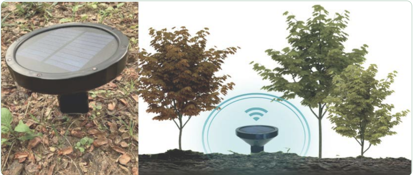
▲ Soil sensors measure moisture and nutrients and transmit the data to the irrigation control system.
