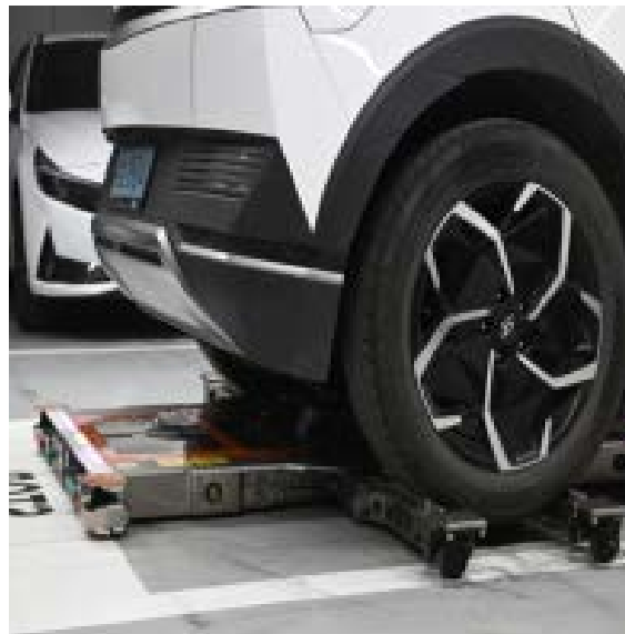
A parking robot goes under a vehicle to lift it up and move it
