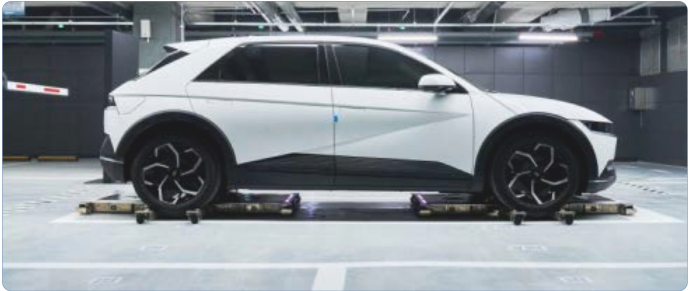
▲ An autonomous mobile parking robot is positioning a vehicle into an available parking spot.
