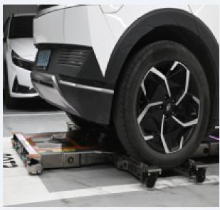
Parking Robot Entering Under the Vehicle to Lift It
