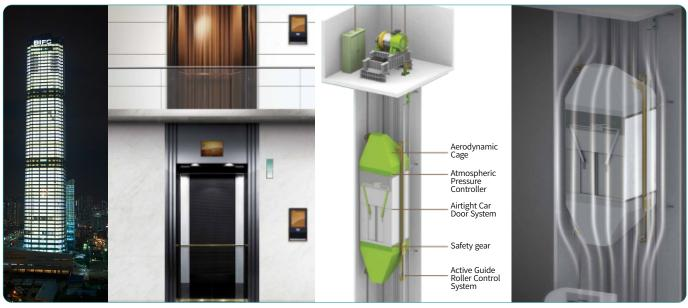
▲ The cable-type capsule in high-speed elevators minimizes operating noise.
