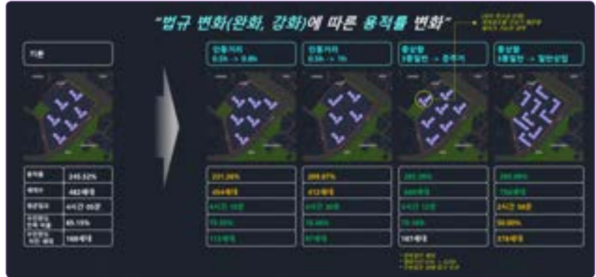
Figure 5 AI-Powered Design Outputs Based on Variations in Setback Distance and Zoning Parameters(BUILDIT)
