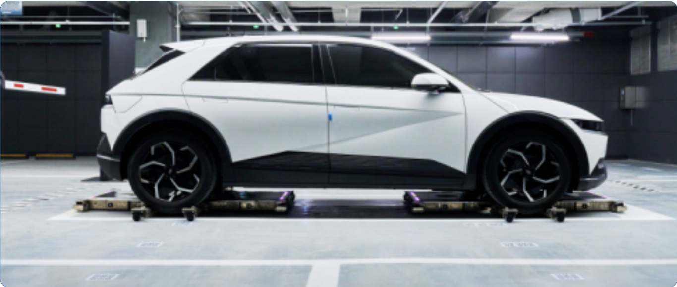
▲ An autonomous parking robot moves a vehicle into a parking space.
