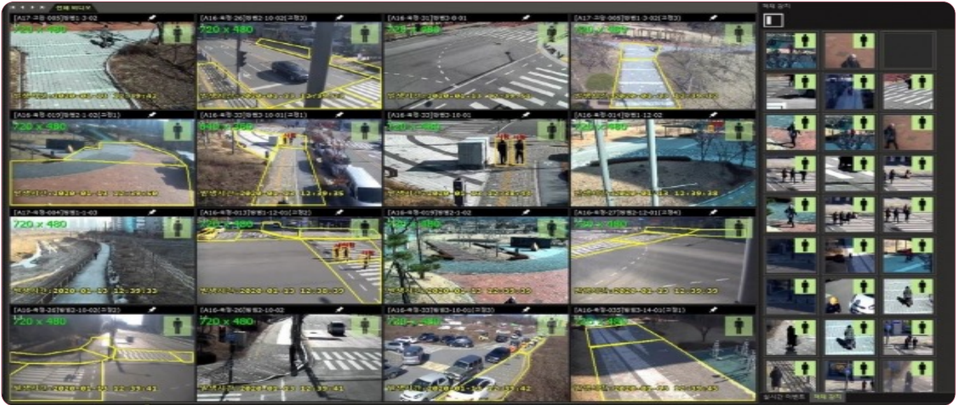
▲ The system analyzes CCTV footage, recognizing and categorizing spaces, objects, and individuals.
