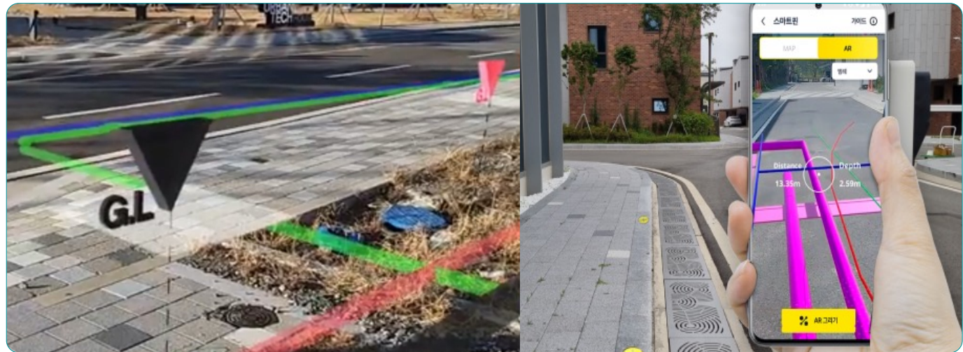
▲ The facility manager is checking the location and attributes of 3D underground facilities based on augmented reality.
