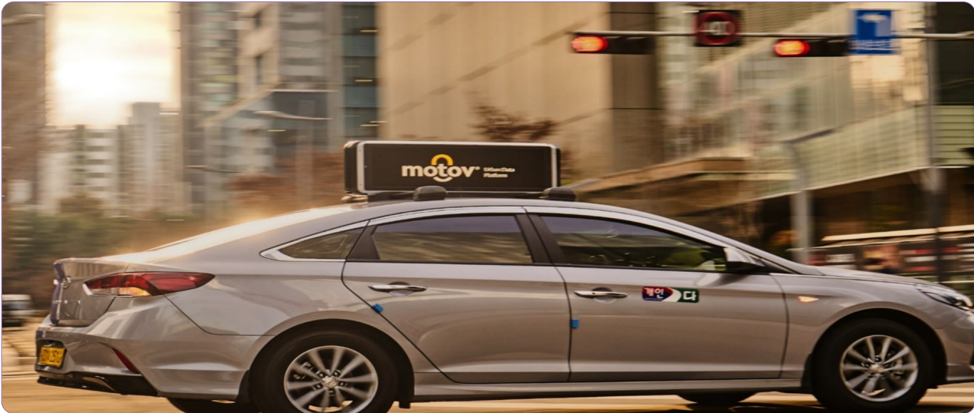
▲ The sensor-equipped device (media board) installed on the taxi roof collects urban data.
